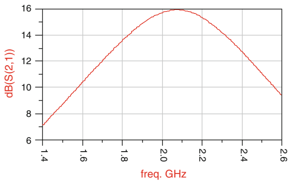
Fig. 14.19 ADS simulation results of S21 of the multistandard LNA, using PSO results
