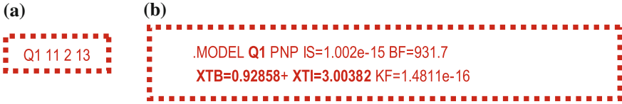
Fig. 7.7 Declaration of one of the two transistors in the op-amp SPICE model
