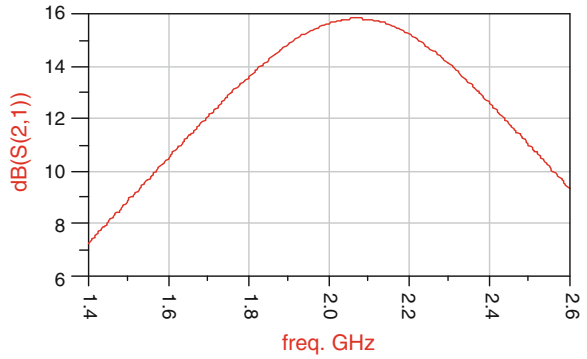
Fig. 14.23 ADS simulation results of S21 of the multistandard LNA, using BSA results
