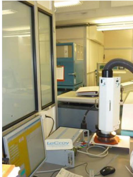
Fig. 7.4 Experimental apparatus for measurement and test of op-amp performances
