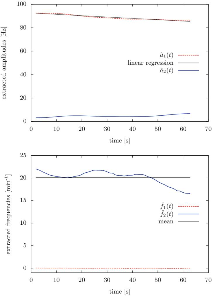
**Fig. 3** Demodulated amplitudes and frequencies from the MFA signal of Fig. 2. The linear regression of  $\hat{a}_1(t)$  and the mean of  $\hat{f}_2(t)$  are also shown as they are used to obtain a compact representation of fatigue and cadence for the overall exercise
