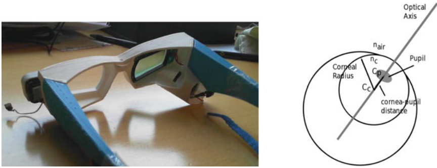
Fig. 1 Left: Prototype of the gaze tracking glasses of [13]. Right: A simplified model of the human eye. C_c and C_p refer to corneal and pupil centers; n_{air} and n_c refer to refractive indices of air and cornea
