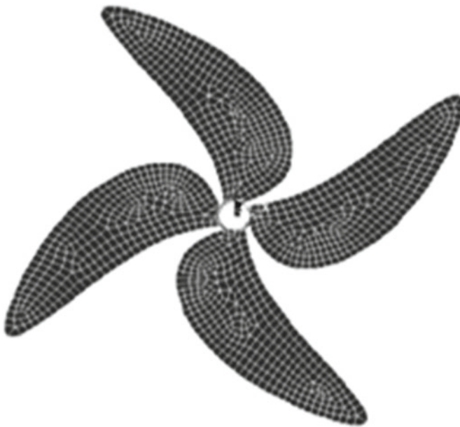
Fig. 3 Finite elements discretization of this immersed structure
