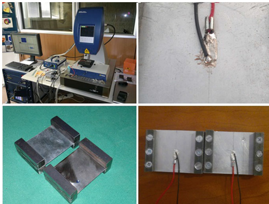
Fig. 2 Experimental layout (clockwise from the upper left corner ): Polytec scanning laser vibrometer, piezoelectric actuator, undamaged and damaged 50 mm \times 50 mm aluminum and steel plates (thickness equal to 0.5 mm). The plates have clamped boundary conditions on two sides and free conditions on the other two sides. Damage is introduced by halving the plate thickness within a circle having 2 mm diameter and the center about 14 mm far from one corner
