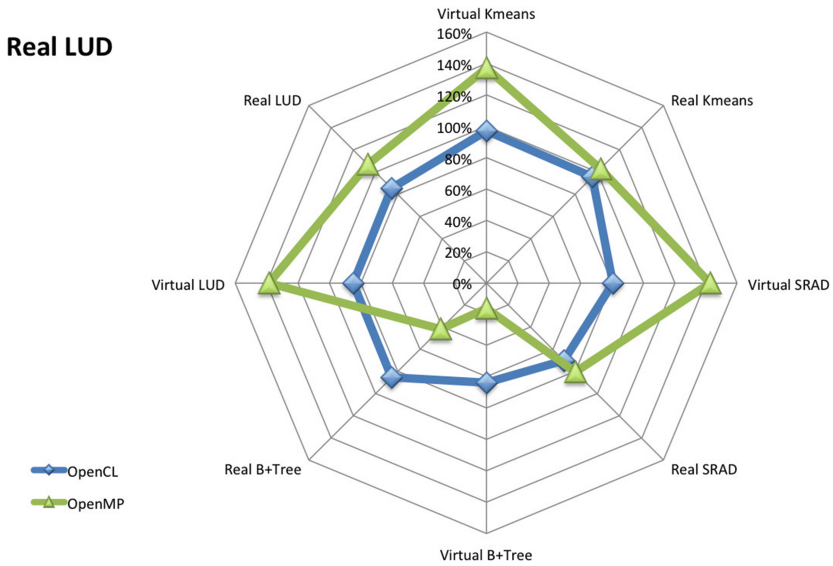
Fig. 2. Performance loss value of the LUD application algorithm executed in a real environment, caused by the concurrency of LUD or B+Tree or Kmeans or SRAD running in a real or virtual environment.
