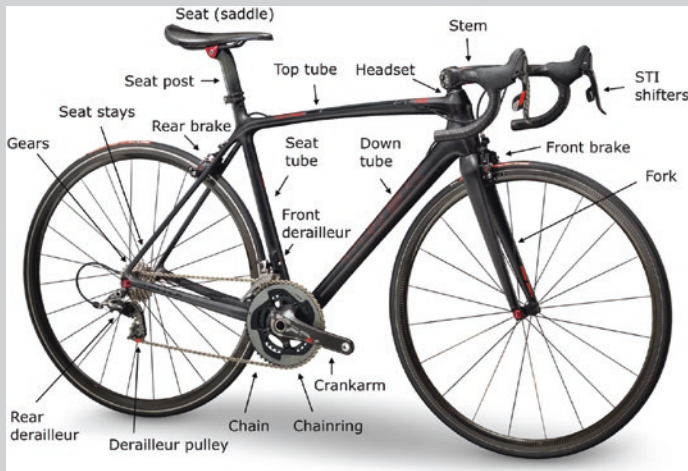
Fig. 8.10 Bicycle terminology, courtesy Daniel Barreneche
