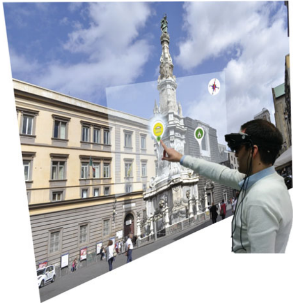
Fig. 1 The user's FOV is augmented with a set of POIs, which can be selected via a touchless point-and-click interface
