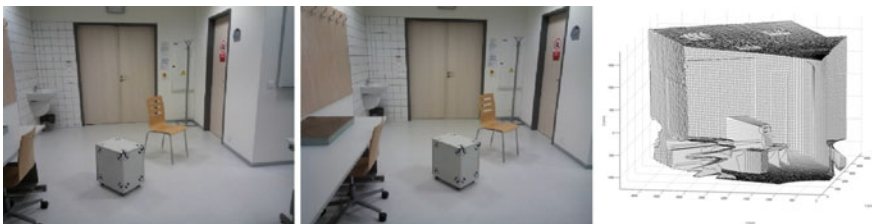
Fig. 1 Experiment input data: Hand-held camera images (left and center) 3D scan of scene (right)
