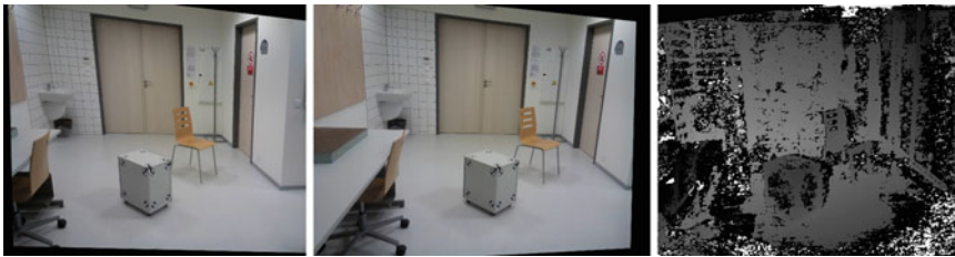
Fig. 2 Rectified images (left and middle), disparity map (right)
