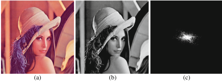
Fig. 2 (a) Colour image. (b) B&W image. (c) FFT application to image (Colour figure online)
