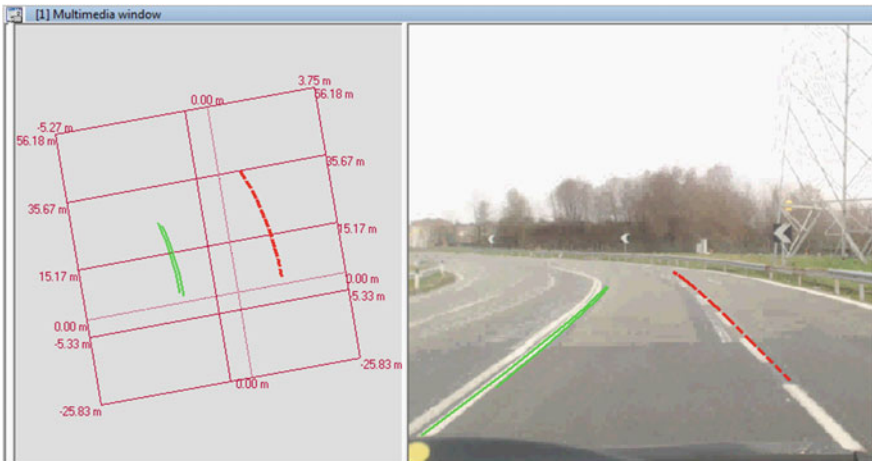
Fig. 15 LDW ECU bird and video display
