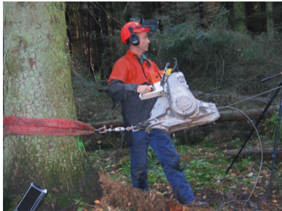
Fig. 2.6 Static tree-pulling with motorized winch to determine critical turning moment (photo credit J.-C. Ruel)
