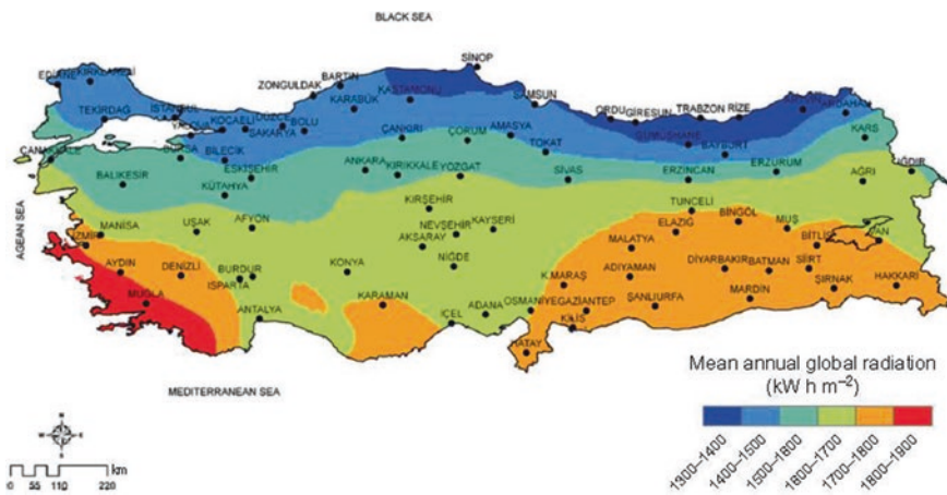
Fig. 4 Geographical distribution of 22-year average of annual global solar irradiation based on NASA/SSE (Aksoy 2011)
