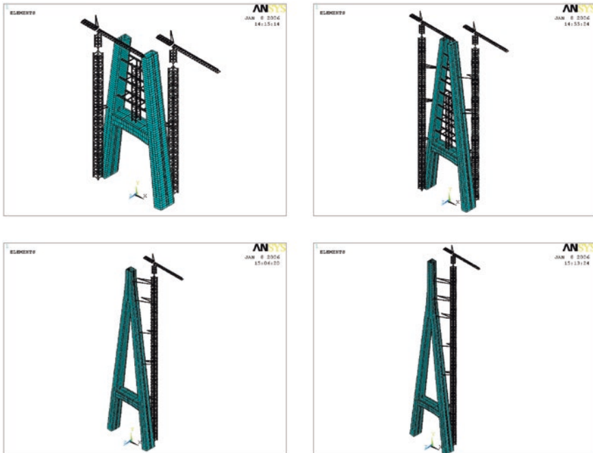
Fig. 6 Construction process of the pylon of Sutong Bridge
