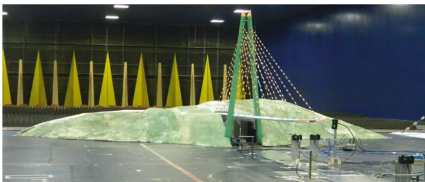
Fig. 7 Aeroelastic model of the cantilever deck construction stage of the BB3 in the POLIMI wind tunnel with turbulent flow conditions
