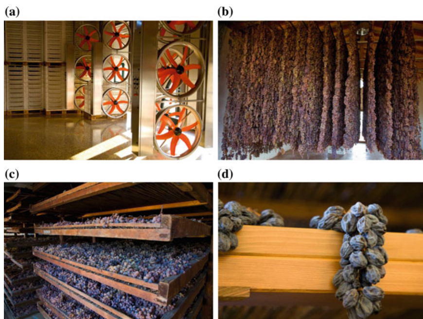
Fig. 1 a Automatized chamber to dehydrated grapes; (b, c) traditional methods applied in Italy to dehydrate; d grape appearance during the process [30]
