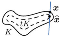
Fig. 1.6 Estimating \mathbf{x} by blowing up K until it touches the affine subspace \{\mathbf{x}' : A\mathbf{x}' = \mathbf{y}\}
