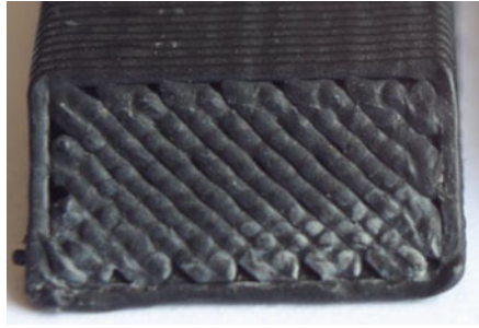
Fig. 1 View of a single layer of a sample manufactured by FDM technology – visible contour and filling threads (thread width approx. 0.5 mm, layer thickness 0.254 mm)
