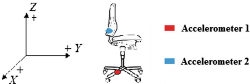
Fig. 1 The placement of the accelerometers in the chairs and the directions of the axes
