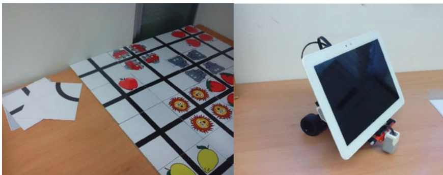
Fig. 2 The tangible surface's parts. On the left, the different tiles that compose the physical surface. On the right, the mobile robot that displays the digital content
