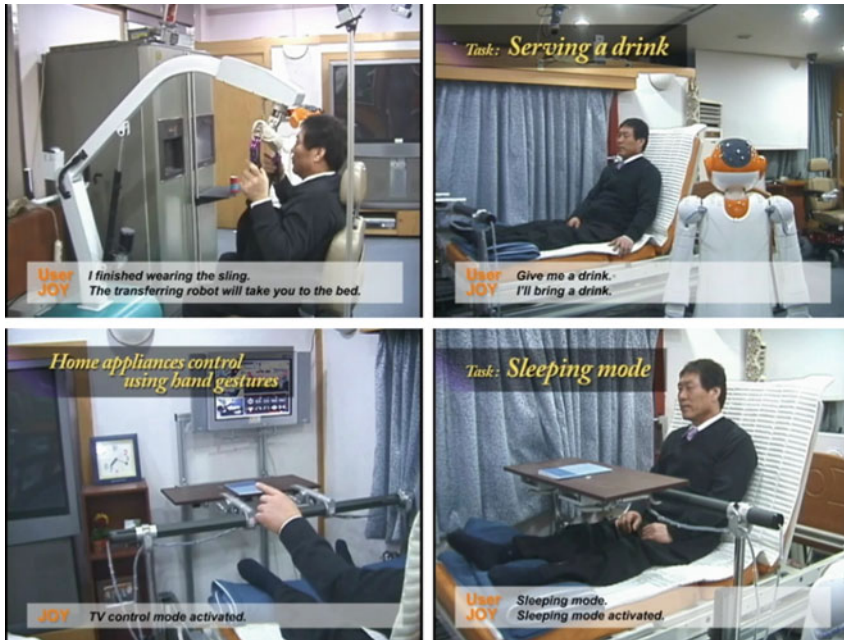
Fig. 2 KAIST's intelligent sweet home scenario. Multiple agents interact to provide a user with disabled lower-limbs a variety of proactive services, which consists of multiple low-level commands carried out by a transferring robot (shown in the upper left), a steward robot (shown in the upper right), a hand gesture-based soft remote control system (shown in the lower left), and an intelligent bed with a robotic arm (shown in the lower right)
