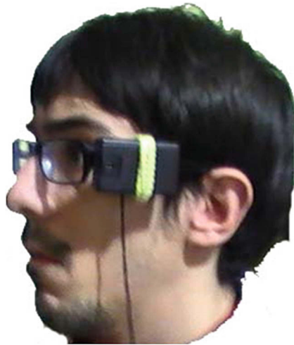
Fig. 2. A wireless accelerometer-based sensor node attached on the head. In this case, it is connected to the Arduino Yun wirelessly.
