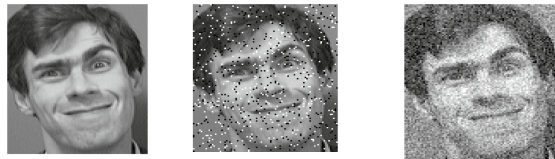
(a)Salt&pepper Noise (b) Gaussian Noise (c) Gaussian Noise m=0, v=0.01 m=0, v=0.04
