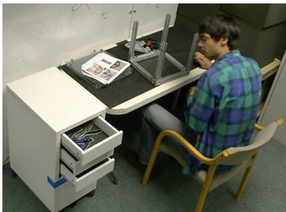
Fig. 5 Emotive drawers performing an animation gesture while a human collaborator assembles a cube puzzle
