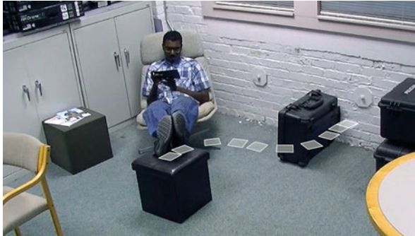
Fig. 3 A typical path taken to approach a seated person. Squares represent the ottoman’s position, one second apart
