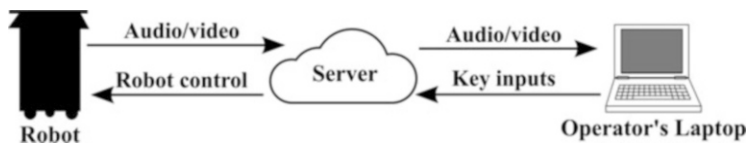
Fig. 9 The roving trash barrel robot’s control system. Cameras on the robot send video to a remote operator’s interface on a laptop, which sends motion commands back to the robot
