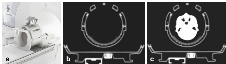
Fig. 1.4 Attenuation correction PET/MR hybrid imaging. Photograph (a) shows a head/neck radiofrequency coil that was optimized for PET transparency for use in an integrated PET/MR hybrid system. Image (b) shows a transversal view through the CT-based hardware attenuation map of a PET/MR system's patient table with a radiofrequency head coil in place. In image (c) the MR-based attenuation correction map of the patient tissues (head) has been added. Thus (c) shows the completed attenuation map that represents the geometric distribution of attenuating hardware and soft tissue structures in the PET field of view
