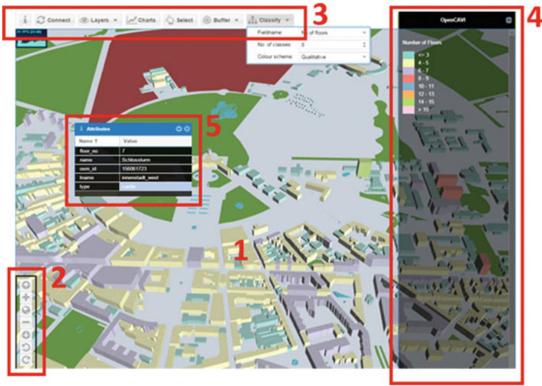
Fig. 6 A 3D web interface layout consisting of Viewer window (1), Navigation controls (2), Toolbar (3), Action panel (4), and Information windows (5)
