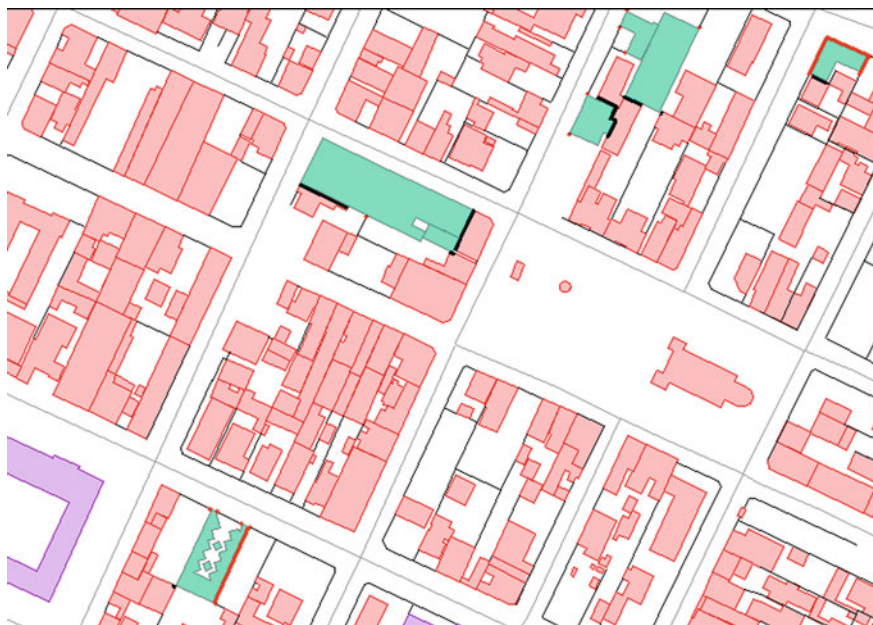
Fig. 14 Black polygons and red lines—legibility problems detected on Campo Largo city topographic map at 1:2000 for better visualization
