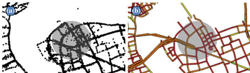
Fig. 4 Examples for selection areas in a global view with a FCD records as points and b classified road partitions
