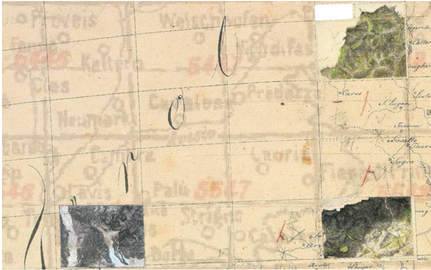
Fig. 2 Map-sheets XI.6–7 and XI.10 of the Kriegskarte (right-side) and map-sheet 5546–4 of third military survey (bottom-left; aligned, see text) georeferenced with proposed methodology (adapted by the authors from sources as Fig. 1)
