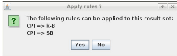
Fig. 2. Charlie asks the user for applying a rule. Charlie handles each property separately. Thus, there is a rule for “k-bounded”, and there is a rule for “structurally bounded” as well, although the property “structurally bounded” implies the property “k-bounded”.
