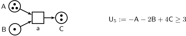
Fig. 5. A net structure S_5 with marking m_5 and an a -sharp inequality U_5
