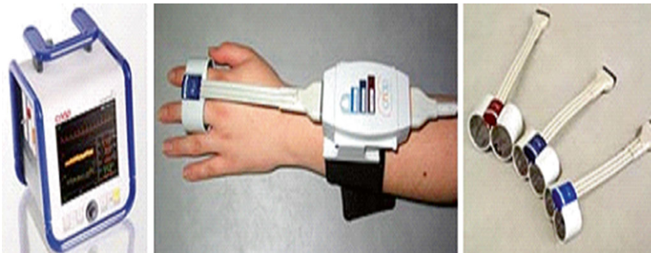
Fig. 23.5 Continuous noninvasive arterial blood pressure (CNAP) provides a continuous, beat-to-beat, blood pressure signal recorded from the fingers of a subject. The monitoring system uses a double finger cuff
