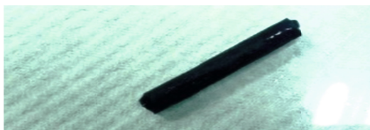
Figure 1. The genipin cross-linked gelatin/cellulose composite scaffold.
