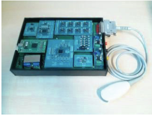
Figure 4. Electronic board for analog front end, FPGA based digital beamformer and 64 element probe.
