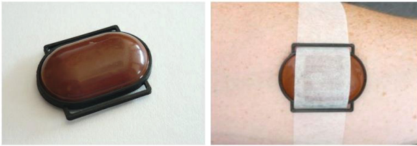
Fig. 3 Temperature sensor and its fixation (right)
