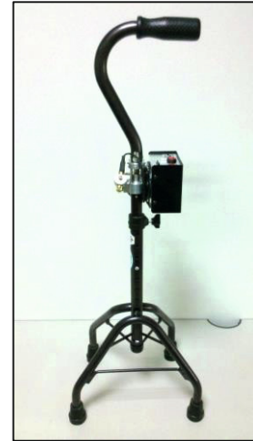
Fig. 1 An early functional prototype of a cane with external cues for stroke patient's gaiting training
