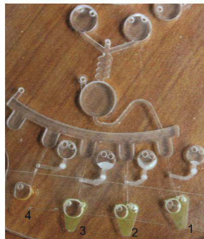
Fig.4 Results of LAMP amplification after adding 1 \mu L of SYBR Green I. The green color determines a positive result, while an orange color indicates a negative result.
