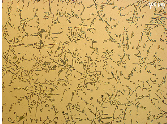
Fig. 4 Microstructure of the cast aluminium AlSi9Cu after aging
