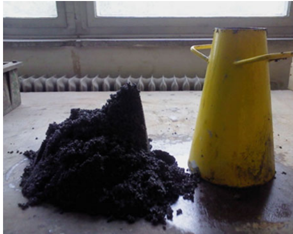
Fig. 6 Shearing failure of cone during the slump test of recipe 1
