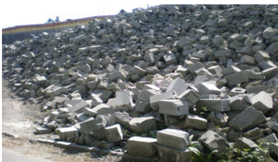
Fig. 1 Waste blocks (rubble) from the production of autoclaved cellular concrete
