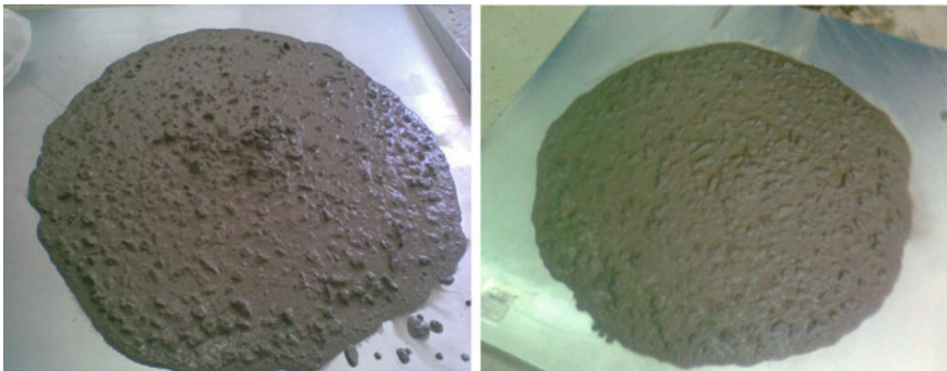
Fig. 6 Slump-flow test: the mixtures C1S5 (left) and C1S10 (right)
