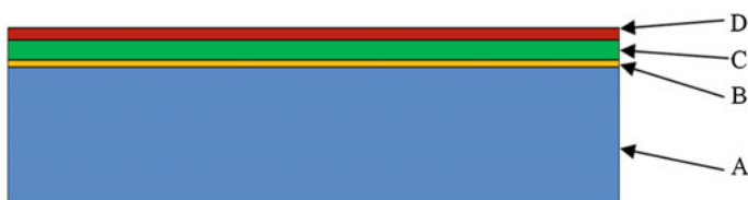
Fig. 1 Schematic diagram of the geometry of the samples of the cast magnesium and aluminium alloys with the deposited coatings onto the surface, where: a substrate, b intermediate layer, c gradient layer, d outer layer
