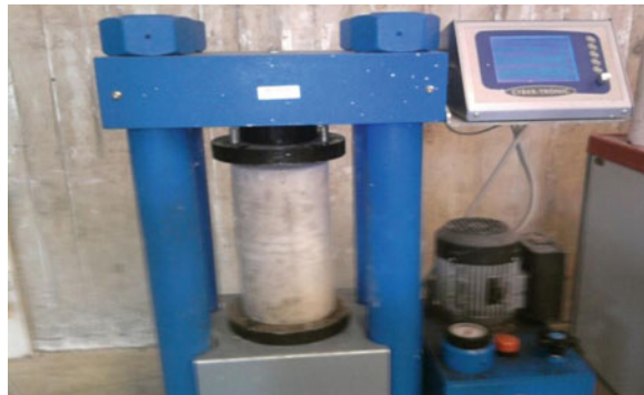
Photograph 1 Compression test set up
