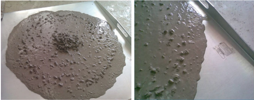
Fig. 5 Slump-flow test: the mixtures C3S10 (left) and C3S5 (right)
