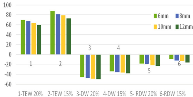
Fig. 5 % Discrepancies between Scatter Correction Methods and simulated total scatter vs. tissue's thickness
