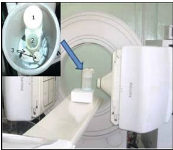
Fig. 1 Philips Forte Gamma Camera with pinhole collimator, neck-thyroid's phantom used to MC simulation and verification, ^1 Spine, ^2 Trachea, ^3 Thyroid
