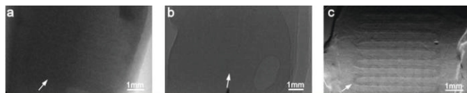
Fig. 5 X-ray images of the polymer scaffold embedded in rat muscle tissue: (a) laboratory-based radiograph at 60 kVp, (b) PCI image at 20 keV, and (c) DEI image at 20 keV. Arrows in (a), (b), and (c) indicate the location of the scaffold in the muscle tissues [19].
