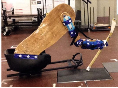
Fig. 1. An illustration of the anatomically correct average adult male wood prototype designed to investigate the preparation phase for shoulder joint produced seated locomotion (not test position).
