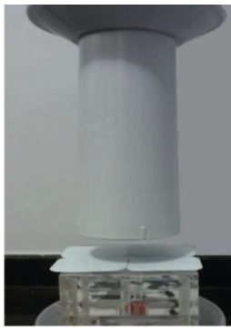
Fig. 1 Phantom of high and low contrast and all dental X-ray.
