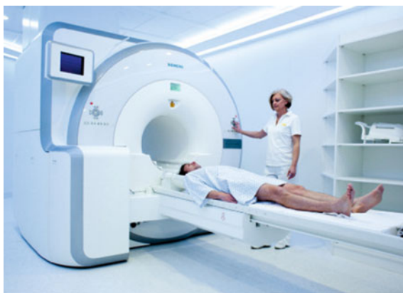
Fig. 10.12 The Biograph mMR scanner made by Siemens can simultaneously carry out MRI and positron emission tomography (PET). It is the first of its kind and was approved in 2010. Source Courtesy of Siemens AG
