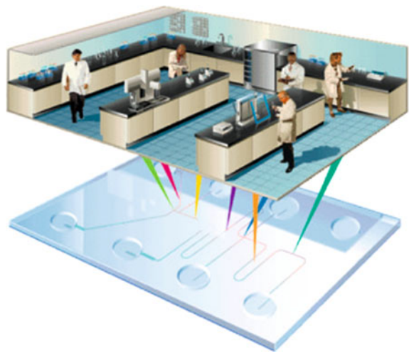
Fig. 10.8 The lab-on-a-chip can carry out the same work as a conventional laboratory for biological analysis, but on an area 1,000,000 times smaller. Source From the French biotechnology site www.biorigami.com
