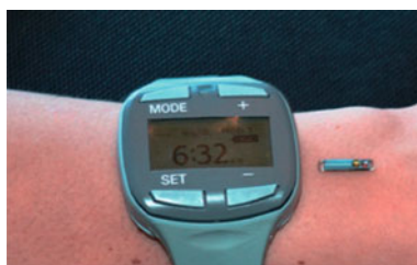
Fig. 10.16 Non-invasive glucometer. Glucose is extracted through the skin by reverse iontophoresis, i.e., extraction of electrically charged molecules from a biological medium under the effects of an electric current. It is then detected by an amperometric biosensor. From [5]
