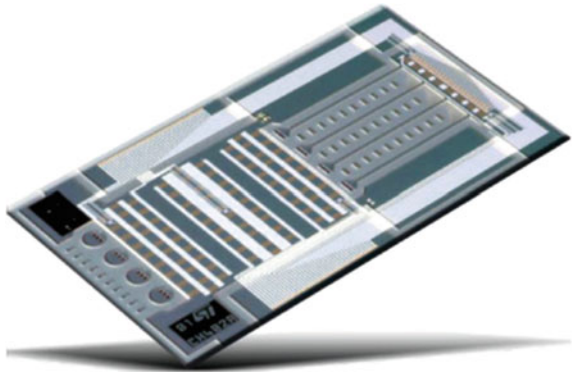
Fig. 10.10 Lab-on-a-chip. Integrated analysis system InCheck. Length 20 mm. Source STMicroelectronics
