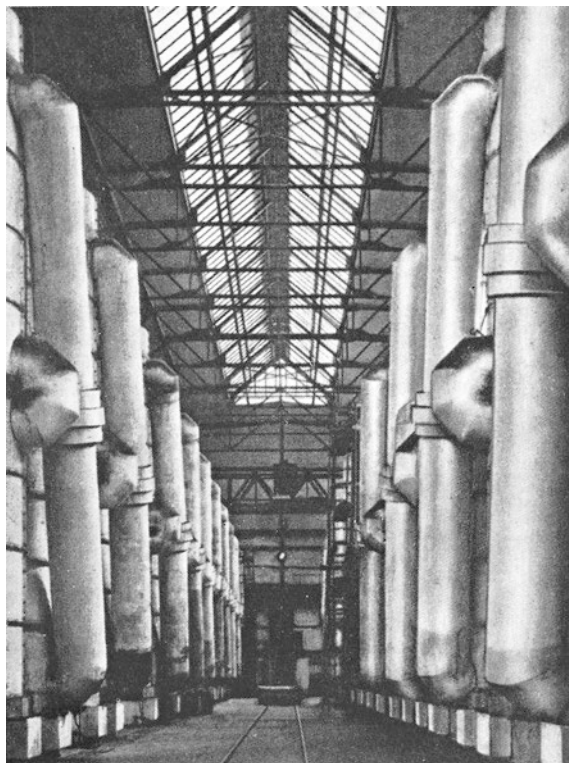
Fig. 4.7 Ammonia synthesis, BASF Merseburg/Leuna. (Tongue [43], Fig. 221. I.G. Farben photograph)
