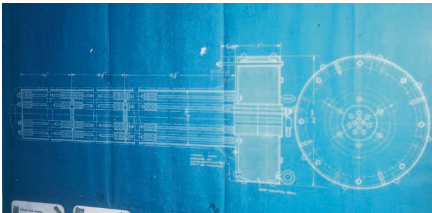
Fig. 3.3 Blueprint of vessel for Chaim Weizmann's fermentation process used in the production of acetone during World War I. (Photo by author, Weizmann Institute of Science, 1985)
