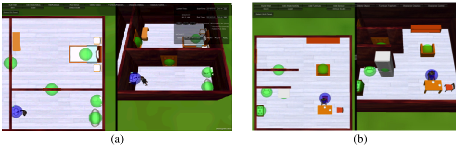
Fig. 2. Screenshots of activity playback. (a) The virtual character is performing Eating breakfast activity in the kitchen. (b) The virtual character is performing Using bathroom activity in the bathroom. Green circles represent sensors with their detection range. When a sensor is triggered by the virtual character, its color changes to purple.
