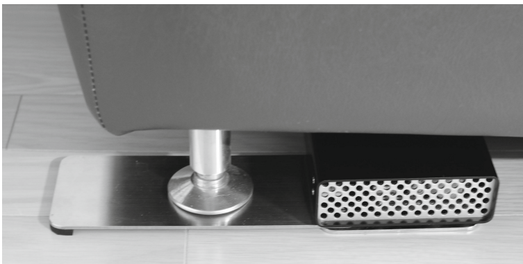
Fig. 3. Proposed Sensor Installed Beneath the Bed Leg
