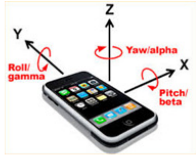
Fig. 2. The X, Y, Z, axes of a mobile phone. Source: http://hillcrestlabs.com
