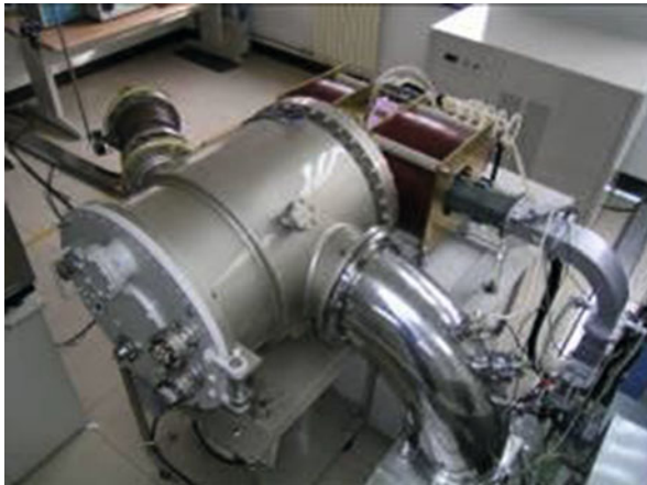
Fig. 4 Photo of atomic oxygen simulation facility
