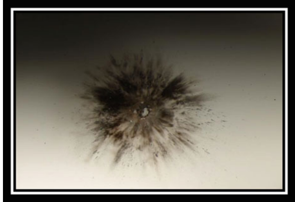
Fig. 3 Space debris impact on optical glass
