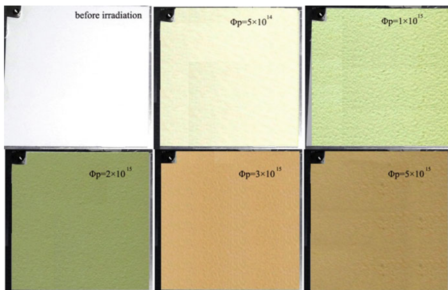
Fig. 3 Surface morphology of the samples before and after irradiation
