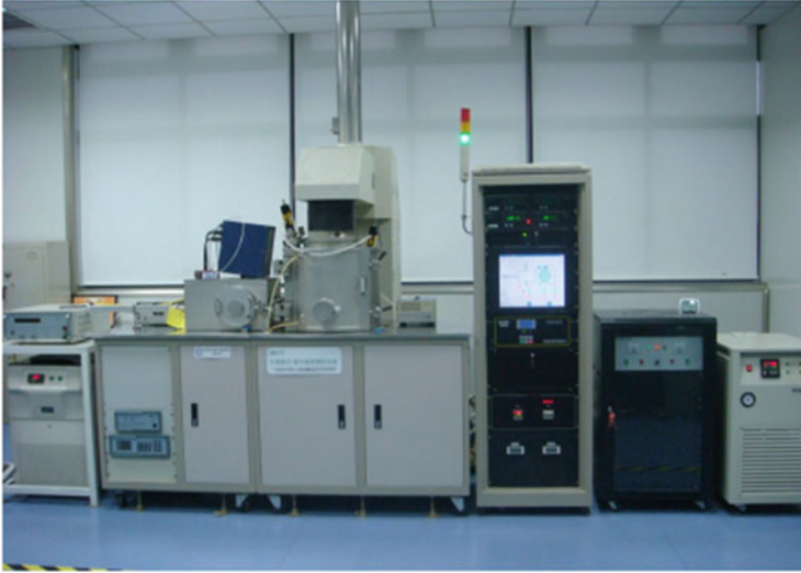
Fig. 1 Long-term ultraviolet radiation exposure facility
