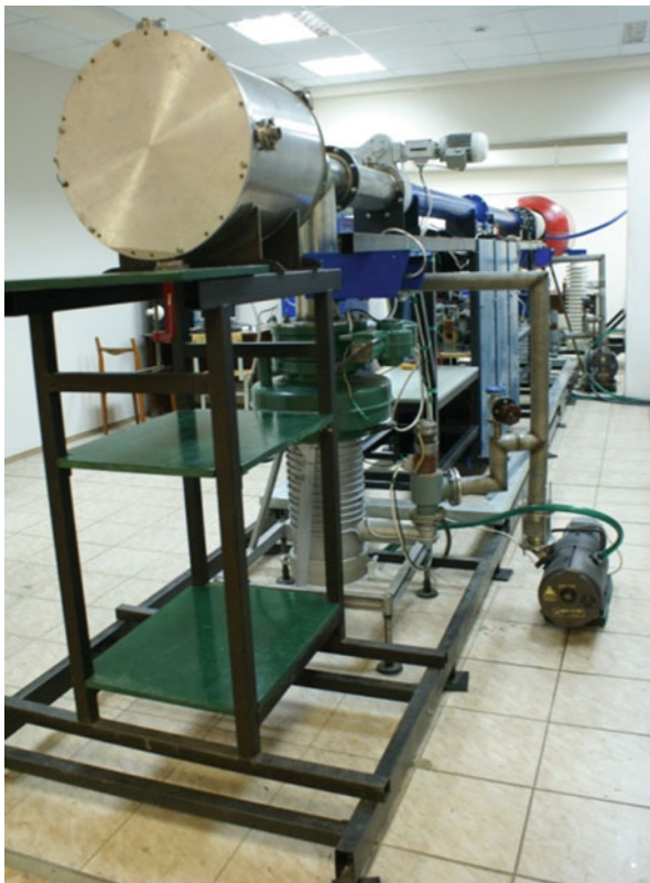
Fig. 4 Accelerator system for simulation of hypervelocity particles [6]. Key Features: Effective accelerating voltage: \sim 735 kV; Particles velocity 15 km/s; particles mass: 10^{-12} – 10^{-15} g
