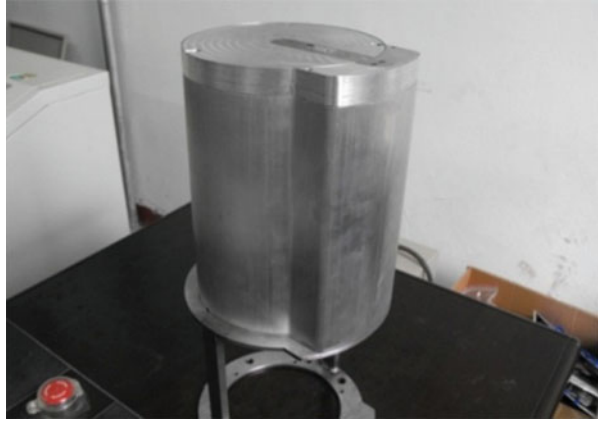
Fig. 3 The automatic packaging and sealing device for transportation of lunar samples developed by Lanzhou Institute of Physics
