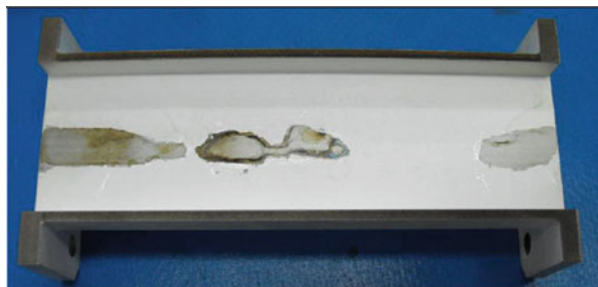
Fig. 5 After the thermal shock test: large plating detachment
