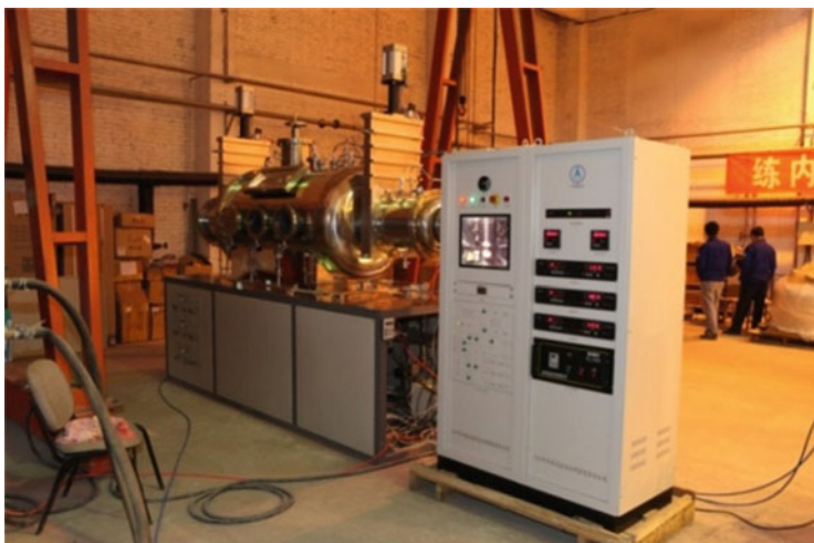
Fig. 4 The device for storing and handling back samples, which could maintain a certain environment for contamination prevention
