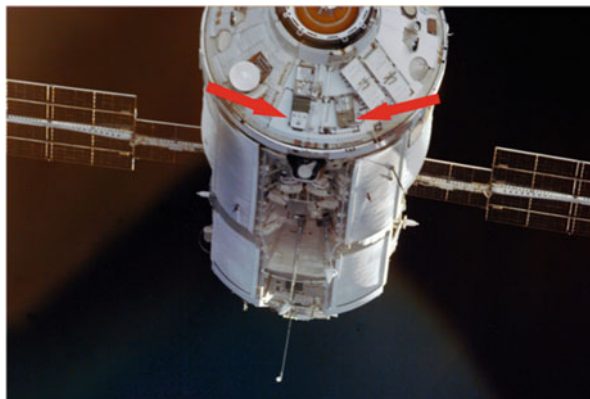
Fig. 1 FGB with mounted Komplast panels 2 and 10, 1998
