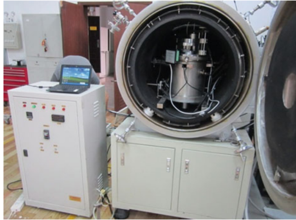
Fig. 2 Lunar dust sediment and adsorption environment simulator
