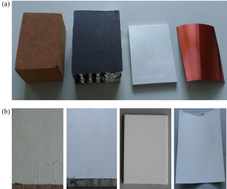
Fig. 3 The samples before and after the thermal cycling experiment: (a) different kinds of substrates, (b) the appearance of the coatings samples after thermal cycling experiment
