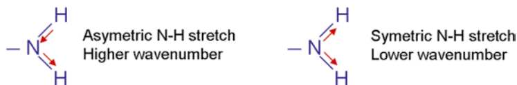
Fig. 7.6 Asymmetrical and symmetrical N-H stretch in primary amines. The N–H stretches of amines are in the region 3300–3000 \text{cm}^{-1} . In primary amines ( \text{RNH}_2 ), there are two bands in this region, the asymmetrical N–H stretch and the symmetrical N–H stretch
