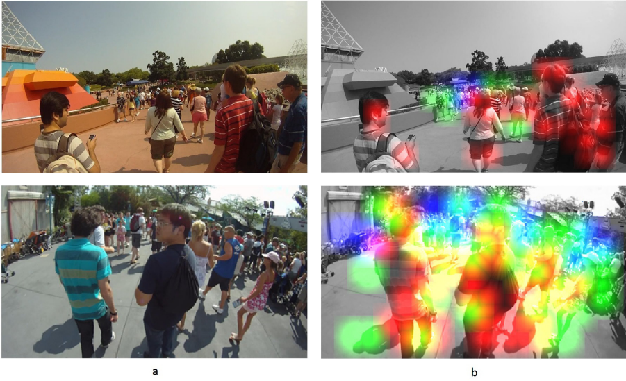
Fig. 4. Examples of crowd detection, the three classes are represented with different colors, from Red for crowds close to the camera, “Crowd” class, to “Far crowd” in blue. In a, the original frames and in b the respective visualization of the crowd’s detection
