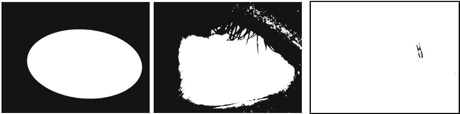
Fig. 5. Ellipse-shaped mask ( M_{ellipse} ), thresholded image in order to get rid of the lashes ( M_{lashes} ) and thresholded image in order to get rid of the shine ( M_{shine} )
