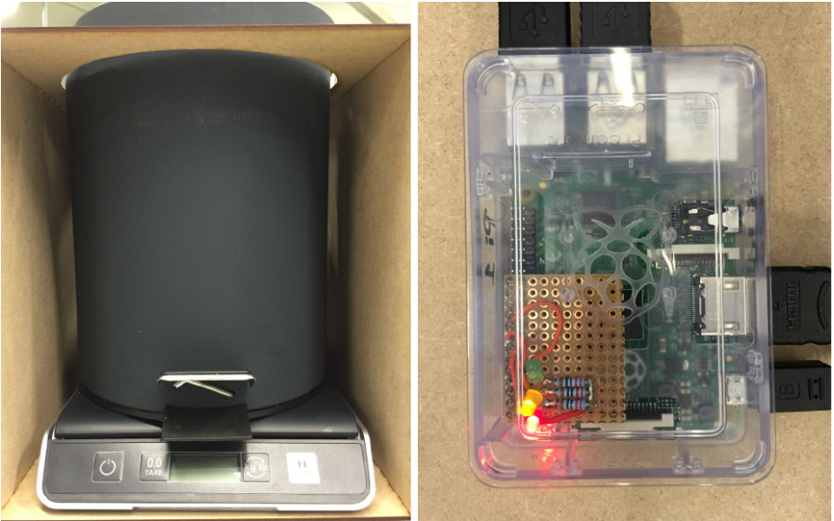
Fig. 1. The bin-scale system of E-COmate with wooden enclosure to protect the Raspberry Pi and to keep the scale and bin fixed. Led lamps indicate when the Raspberry Pi with its program has started (red), when the scale is connected to the Raspberry Pi (orange) and when the Raspberry Pi measured a stable weight and is uploading it to a server.
