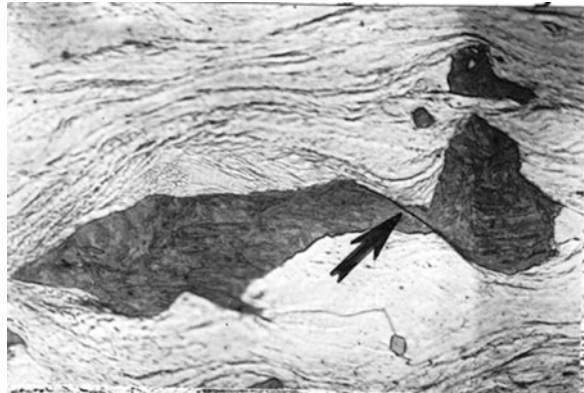
Fig. 3.6 Fracture of martensite grain (indicated by arrow) at heavy deformation OM ×200—original
