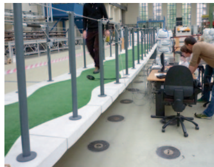
Fig. 6.229 Load-bearing/vibration damping simulation, “walking” on the prototype, TU Berlin
