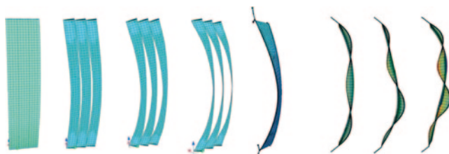
Fig. 6.217 b and c Calculation study of elastically deformed strips
