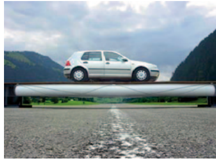
Fig. 6.243 (above right) Tensairity® system
