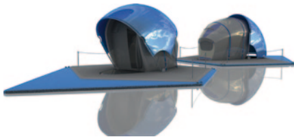
Fig. 6.253 The Physalia floating volumes are drivable with an electric motor
