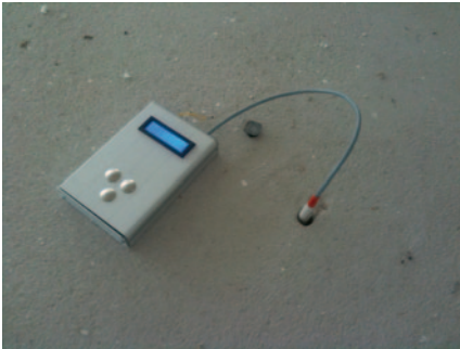
Fig. 6.194 Sensor embedded in cement mortar
