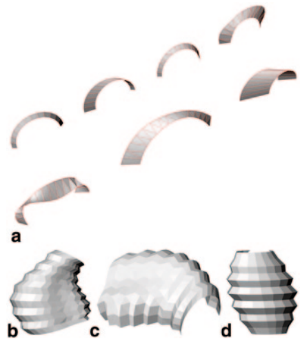
Fig. 6.52 a–e Paper strip models are able to be developed with the aid of triangle structures. The folded masses are more or less irregularly formed and consist of planar individual surfaces, thus easing a technical realization
