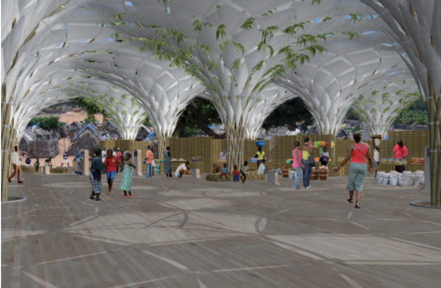
Fig. 6.247 Fully developed bamboo canopy for an outdoor market in a tropical region. The solar membranes serve as Sun and rain protection, lead water to the plant roots, and integrate photovoltaic (PV) modules for solar energy production
