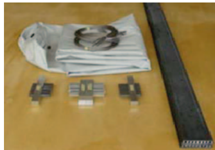
Fig. 6.244 (middle) Components of the Tensairity® system are a long pressure bar, an inflatable membrane for the pneumatic base element, cables for radial and counter-radial tensioning, anchoring parts
