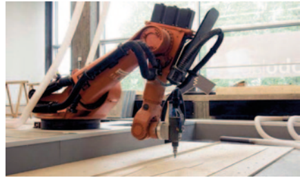
Fig. 6.171 Computer-driven robotic fabrication of the individual plywood strips
