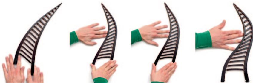
Fig. 6.234 Fin Ray Effect®: Different movement patterns illustrated in model. The number of cross braces is not important for the bending behavior of the entire system
