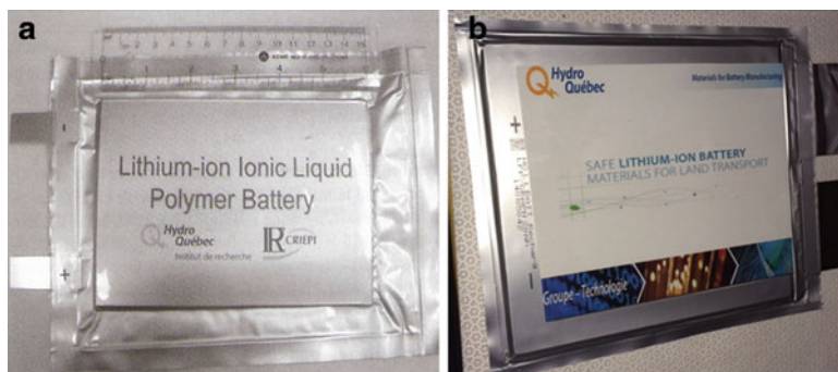
Fig. 15.5 (a) Li-ion flat aluminum bag cell (Ionic liquid/polymer type) with an active surface area of 104 \text{ cm}^2 and (b) prismatic 20-Ah Li-ion cell (A4 format)
