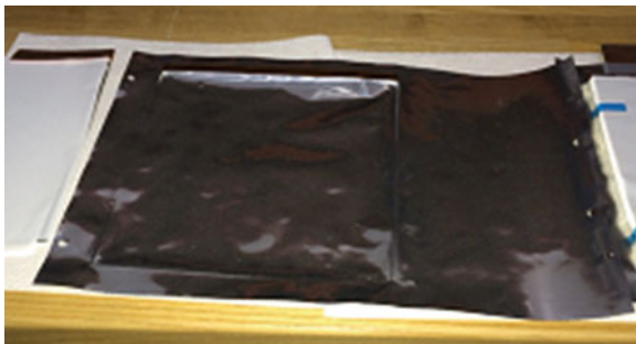
Fig. 15.4 Image of the positive electrode formed by the deposition of the slurry onto an aluminum foil from a reservoir through a slot-die under hydraulic “pump” pressure
