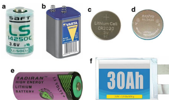
Fig. 2.13 Various battery configurations. (a) LS14250- cylindrical Li//SOCl 2 battery, (b) 4R25-prismatic (container) cell, (c–d) CR2020 Li-MnO 2 coin cells, (e) AA-type Li-ion cylindrical (1.5 Ah, 3.6 V, 12.4 g) cell, and (f) 30-Ah pouch (LiMn 2 O 4 -type, 3.8 V, 850 g) cell
