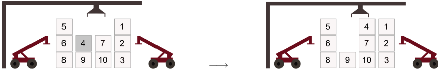
Fig. 1. A container bay with four stacks where the numbers represent the priority values of the containers. Shaded containers are blocked for the gantry crane. The left figure shows the bay before pre-marshalling, the right thereafter.
