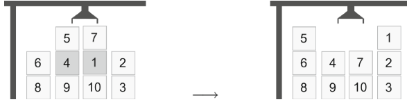
Fig. 1. A container bay with four stacks where the numbers represent the priority values of the containers. Shaded containers are blocked for the gantry crane. The left figure shows the bay before pre-marshalling, the right thereafter.
