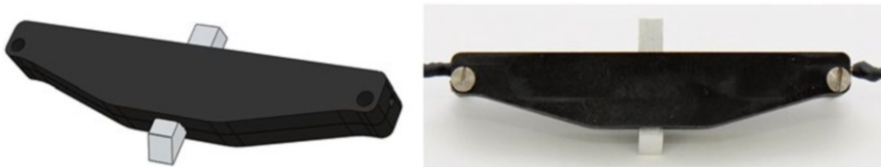
Fig. 4.21 Arc-shaped shape memory alloy actuator for unlocking or valve applications
