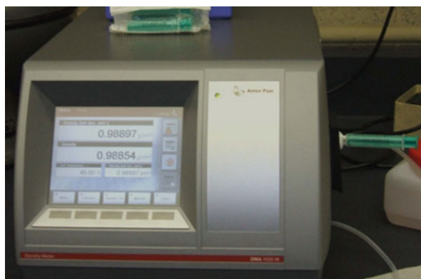
Fig. 2.18 Anton-Paar 5000M vibrating tube densimeter with sample syringe
