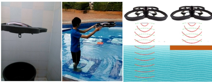
Fig. 5. Closed (left) and open (middle) stations and the water level estimation (right)
