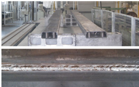
Fig. 5 The rack girder after welding
