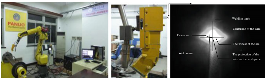
Fig. 24 Welding robot system with visual sensor for monitoring welding pool and tracking seam
