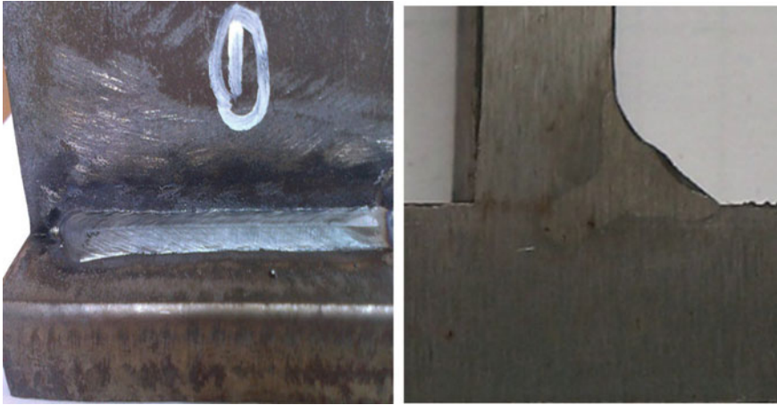
Fig. 5 Macroscopic morphology of laser hybrid welding T-joints (TH-1)
