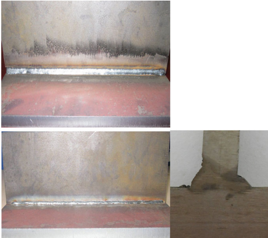
Fig. 7 Macroscopic morphology of laser hybrid welding T-joints (TH-2)
