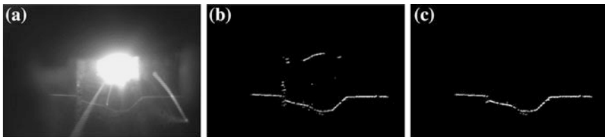
Fig. 7 a The original image with lots of spatter. b The dots in the same positions in the according binary image I and II. c The extracted profile
