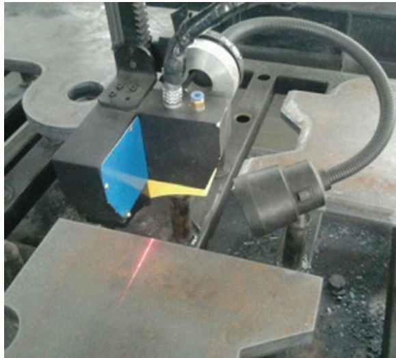
Fig. 2 The prototype of the laser sensor
