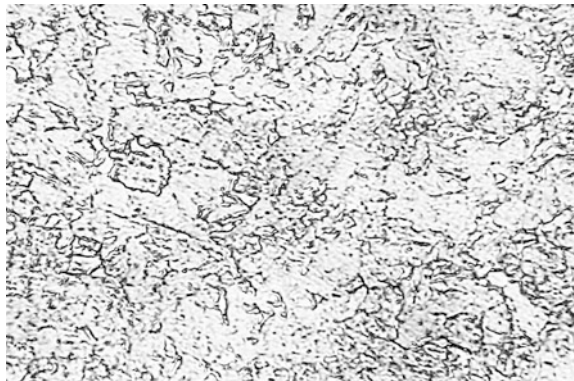
Fig. 10 400× Aqueous solution of ferric chloride (the weld center)
