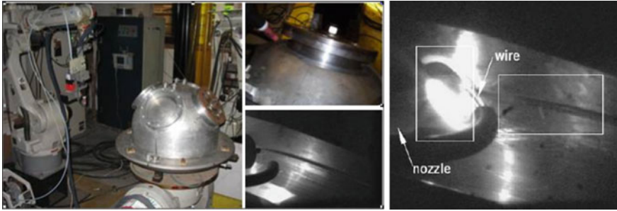
Fig. 27 Application of robotic welding system for real-time control of penetration
