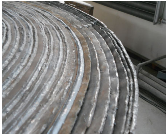
Fig. 7 Overlapped weld seams of spiral board heat exchanger
