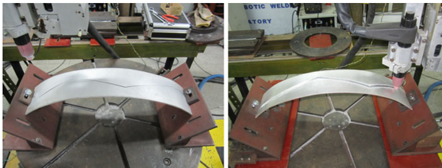
Fig. 26 3D seam tracking results by robotic GTAW system
