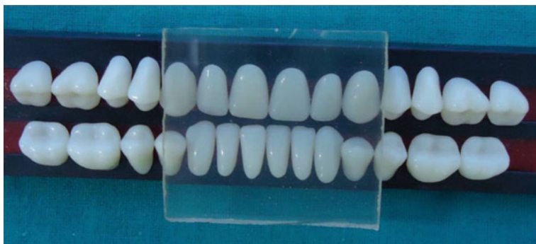
Fig. 10.35 Photographs of a piece of transparent spinel ceramics, together with tooth samples. Reproduced with permission from [182]. Copyright © 2014, Springer Science + Business Media
