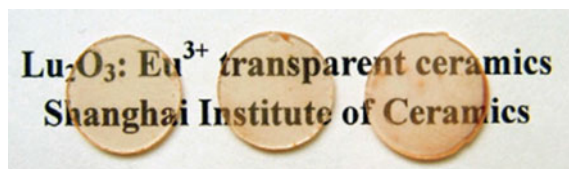
Fig. 2.9 Representative photographs of mirror-polished 5 % Eu 3+ -doped Lu 2 O 3 ceramics sintered at 1850 °C for 6 h, with thickness of 1 mm. Reproduced with permission from [12]. Copyright © 2006, John Wiley & Sons
