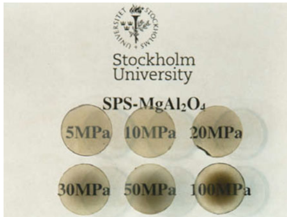
Fig. 7.22 Photographs of the transparent \text{MgAl}_2\text{O}_4 ceramics sintered at 1300 °C for 3 min at different preloaded pressures ( P_1 ): 5 MPa (1.79 mm), 10 MPa (1.99 mm), 20 MPa (1.82 mm), 30 MPa (1.89 mm), 50 MPa (1.82 mm), and 100 MPa (1.60 mm). The samples were 15 mm above the paper, and thicknesses of the samples are indicated in parentheses. Reproduced with permission from [140]. Copyright © 2009, Elsevier
