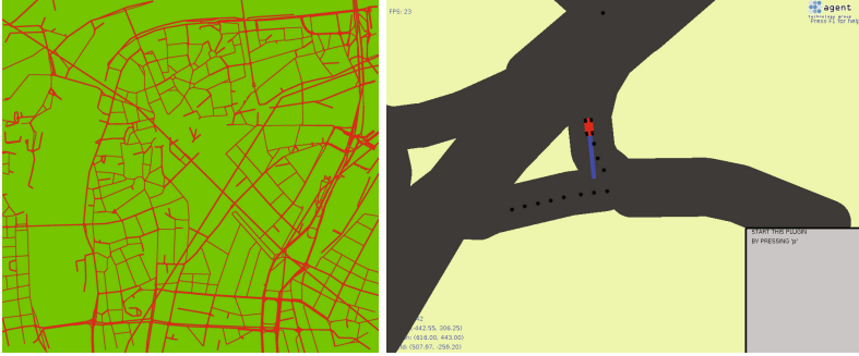
Fig. 2. Visualization of SUMO network data of Prague (left), the red and green image is also used for texturing of the terrain. An example of a bug in data is shown on right, the vehicle is routed to leave a main street to immediately join back instead of just following the main street.
