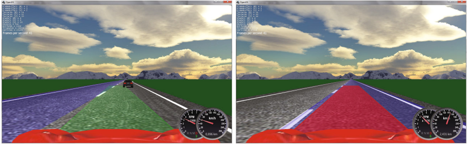
Fig. 6. Driver’s view in OpenDS with integrated HMI for collision avoidance support. The system provides the driver with the visual representation of a proposed plan. The proposed lane to follow is highlighted by blue, the speed adjustment is proposed via green or red signal of appropriate intensity. There is an example of an instruction to change lane to left to overtake (left image). Second case shows how the red color informs the driver of proposal to slow down (right image) because of speeding in this case.
